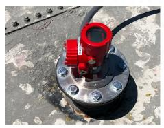
ResinView<sup>®</sup> is compatible with many types of level sensors. Granular, powder, flake, or liquid forms of resin may require different types of sensor technology. Non-contact radars, SmartBobs, and lasers are often used for resin monitoring. No power to the bin, no problem—battery powered sensors make installation easy. ResinView<sup>®</sup> is compatible with sensors using analog or 4-20 mA, Modbus, or HART outputs.
